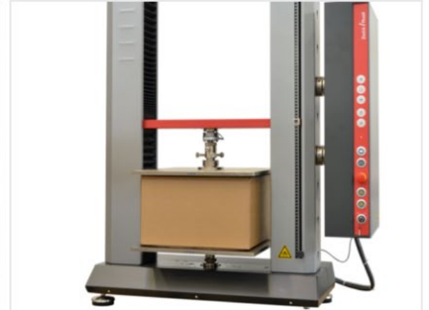
Compression test on packaging
